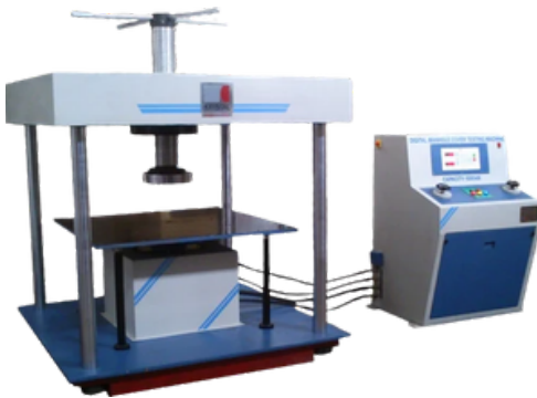
Manhole cover pressure
