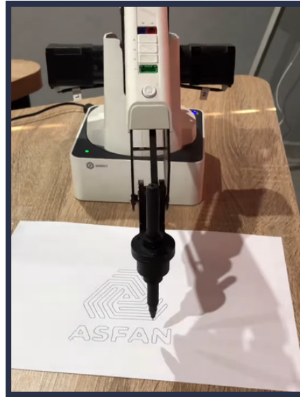
DOBOT – A compact robot arm for teaching programming, robotics, and coordinate control.
